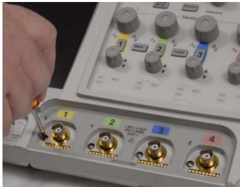
Figure 21 Removing the T6 screws
