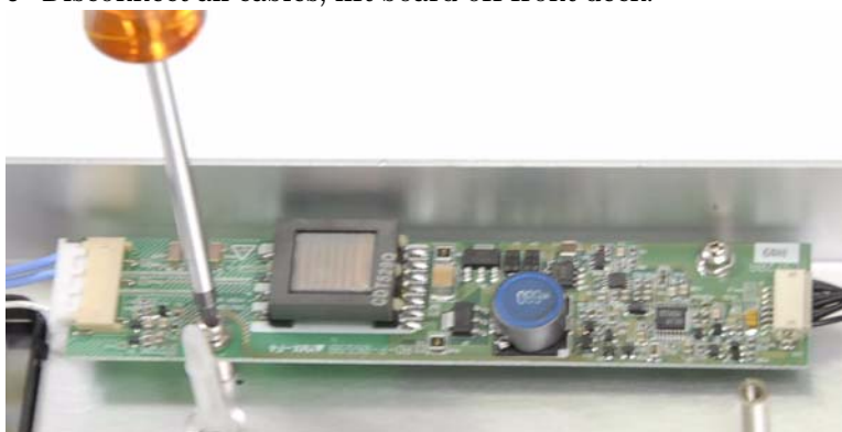
Figure 24 Removal of inverter board
