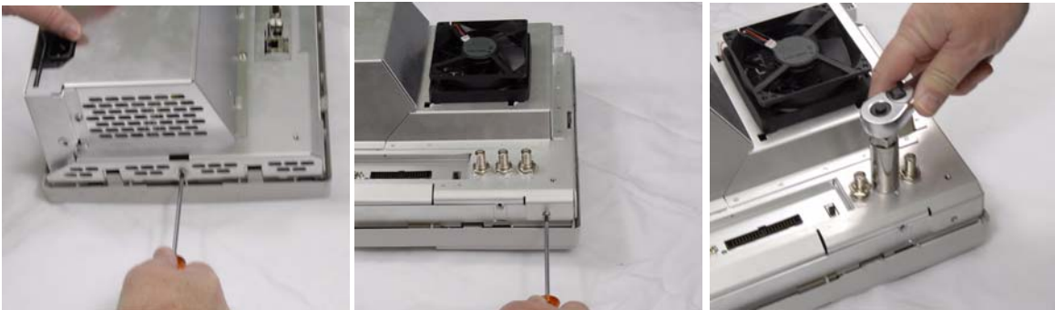
Figure 19 Removing the rear deck assembly
