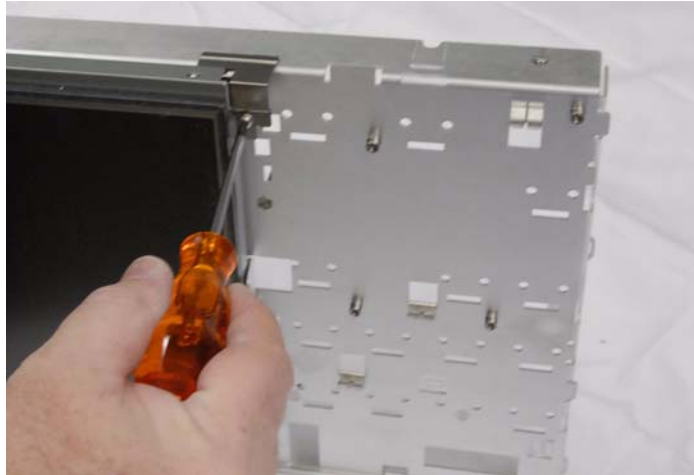
Figure 34 Removing display assembly
