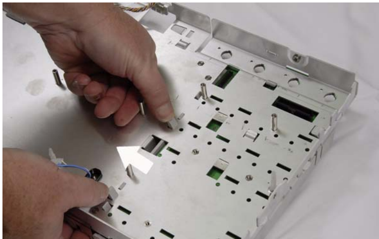
Figure 30 Removing front panel assembly from front deck
