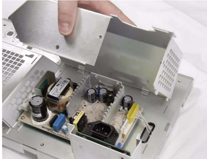
Figure 37 Lifting power supply cover off
