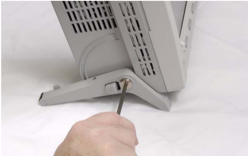
Figure 17 Removing adjustable leg
